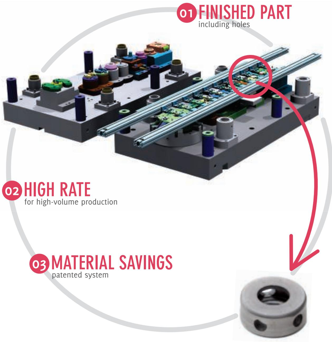
High speed tooling for large volume production of parts which exit the press completely finished, including the holes: a single press is used to perform all operations from coil to finished part.
