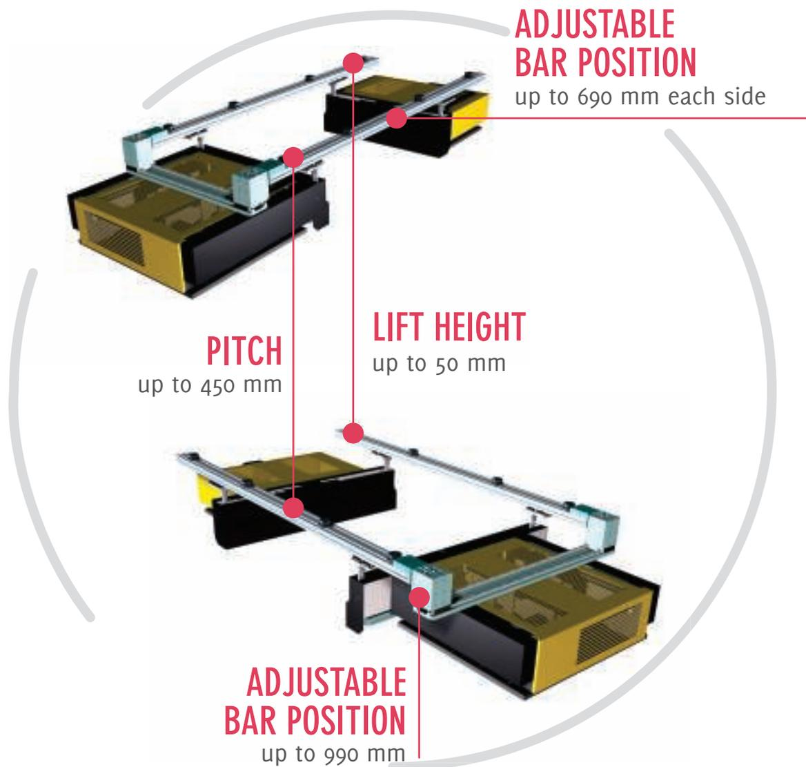
The TE3A series of transfer units combine the features of the TE2A series with the possibility for bar lift motion up to 50 mm. This makes them highly suitable for the production of medium sized parts that require the piece to be lifted during transfer from one station to the next. Just like the TE2A series, the transfer can be located anywhere: installed between the press uprights, set on the press bed, or attached to the upper frame, upside-down.
