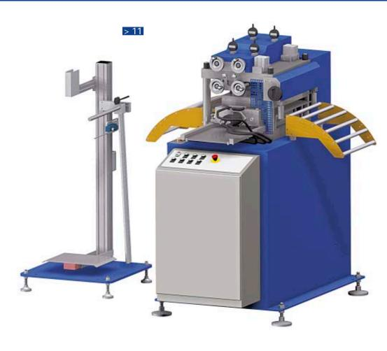
More and more often, the punching industry uses a motorised strip straightener in front of the press. Straightening conserves tools thereby producing more accurate components. As the strip is fed over a loop into the feeder without any pulling force, higher production rates can be achieved.
