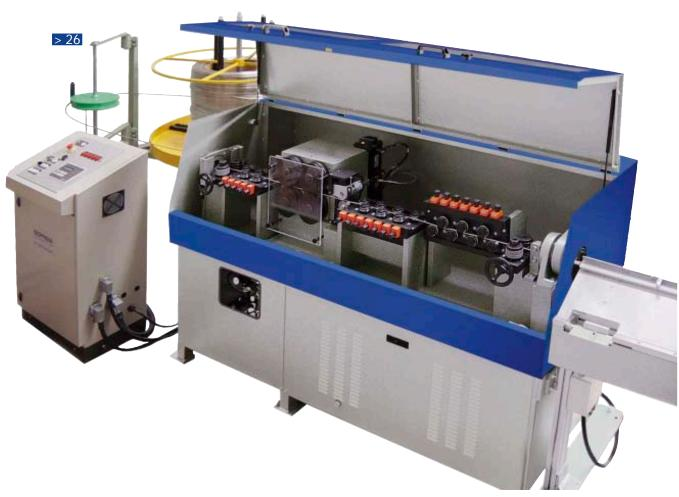
Modern production companies automate wire feeding with decoilers, straightening-feeding systems and cut-to-length lines.
