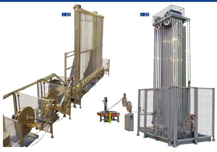
The high productivity requirements in composite pipe production demand strip feeding lines with a strip accumulator system.
